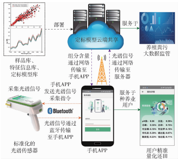
图6 多场景养殖粪污(肥)全养分同步速测系统 Fig.6 Multi-scenario synchronous rapid testing system for total nutrient analysis of livestock manure (fertilizer)
