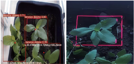
图 16 双目视觉杂草定位结果 Fig. 16 Result of weed localization based on binocular vision
