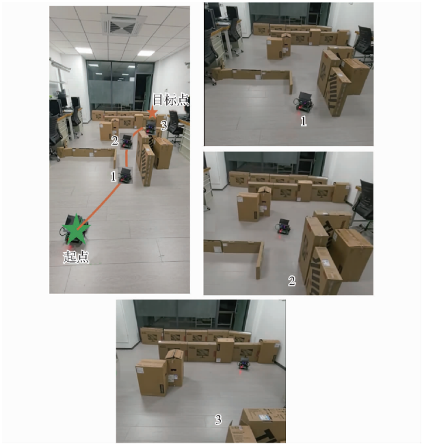
图 13 ROS 导航包默认权重 1 运行实验过程图 Fig. 13 Diagram of ROS navigation package import with default weight-1 operation experiment process
