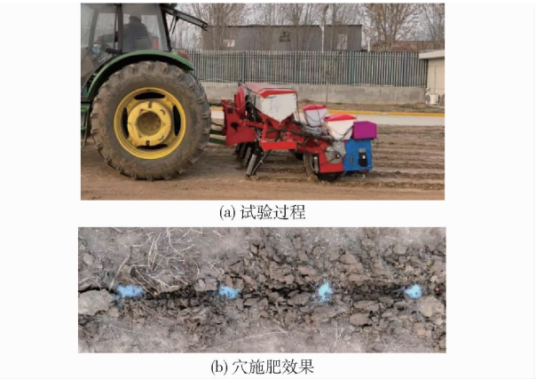
图 17 田间试验过程及穴施肥效果 Fig.17 Field experiment process and effect of hole fertilization
