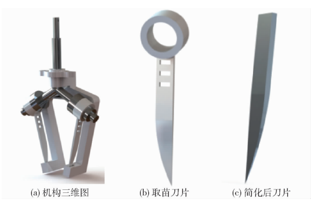
图 3 取苗刀片简化过程 Fig. 3 Simplification process of seedling-taking blade
