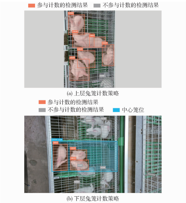
图 6 分层计数策略 Fig.6 Schematic illustrations of layer-adaptive counting strategy
