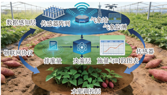
图 17 传感-处方-执行闭环水肥调控架构示意 Fig. 17 Schematic of sensor - prescription - execution closed-loop water and fertilizer regulation architecture
