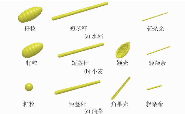
图 5 不同脱出混合物成分颗粒模型(非真实比例) Fig.5 Particle models of different threshed mixture components (non-real scale)
