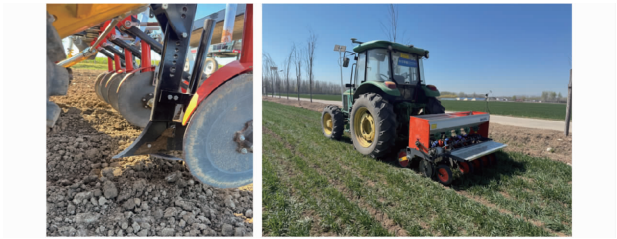
图 25 冬小麦划锄断根施肥机田间试验 Fig. 25 Field trial of winter wheat root-cutting and fertilizer application machine
