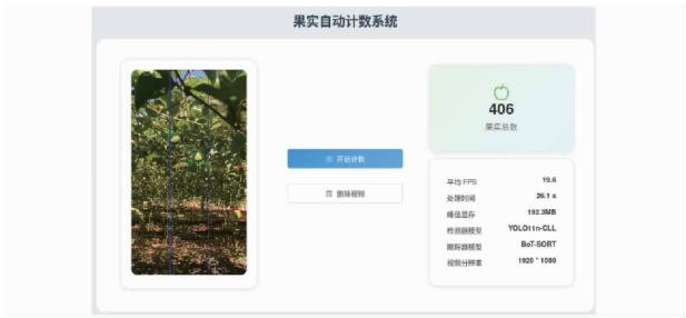
图 13 百香果视频检测、跟踪与计数系统可视化界面 Fig. 13 Visualization interface for passion fruit video detection, tracking, and counting
