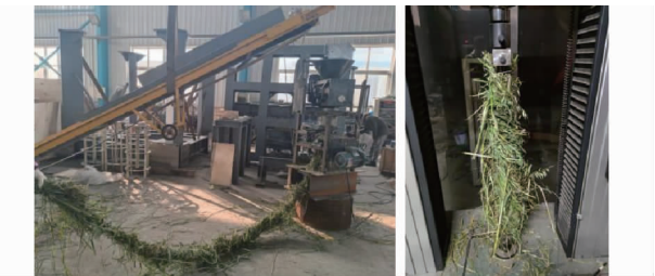
图 9 草辫机加捻草辫试验和万能试验机拉伸试验 Fig. 9 Braiding machine twisting test with straw grass braid and universal testing machine tensile test
