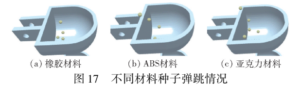
Fig. 17 Seed bouncing for different materials
