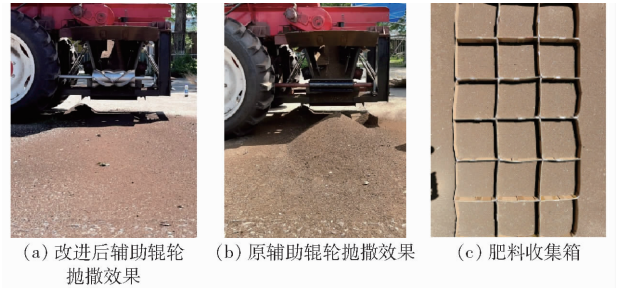
图 21 辅助辊轮创新设计效果检验 Fig. 21 Test on innovative design effect of auxiliary roller
