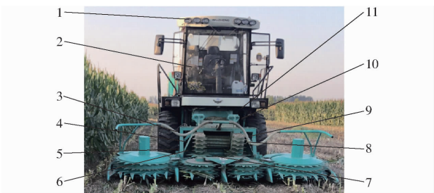
图 8 玉米青贮收获机传感模块机上安装位置图 Fig. 8 On-board installation location of sensors in corn silage harvester
