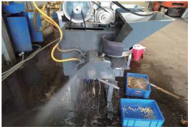
图 14 鲜莲子去皮机试验现场 Fig. 14 Experiment site of fresh lotus seed peeling machine
