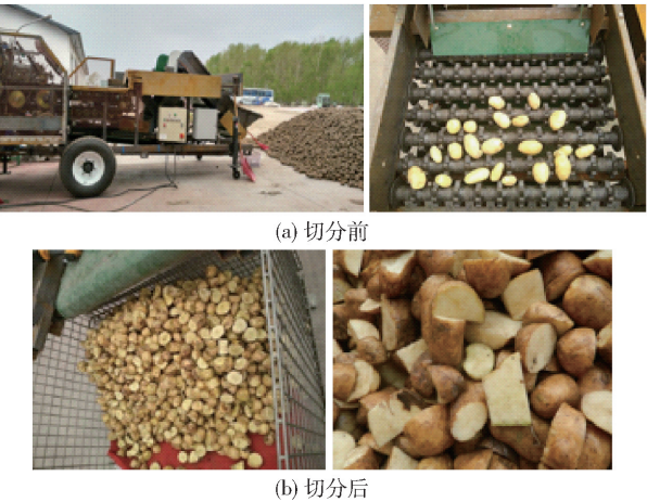
图 19 马铃薯种薯切块机切分前后工作场景 Fig. 19 Working scenarios of seed potatoes before and after cutting machine
