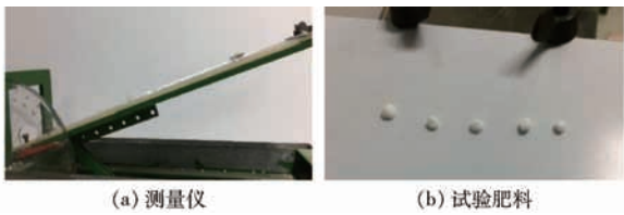
图9 静摩擦因数测量 Fig.9 Measurement of static friction coefficient
