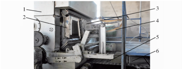
图 10 11SX-800A 型气力式水稻穴盘成型机 Fig. 10 11SX-800A type pneumatic forming machine for seeding-growing tray
