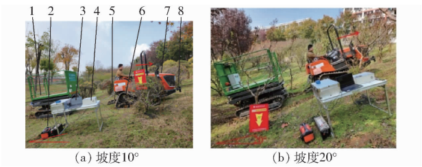
图 16 农夫 NF602 型山地履带拖拉机爬坡牵引性能试验 Fig. 16 Longitudinal traction performance test of Farmer NF602 mountain crawler tractor on slopes
