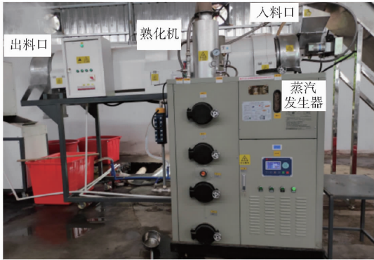
图1 白胡椒初加工生产线熟化环节设备 Fig. 1 Curing stage equipment for white pepper primary processing production line
