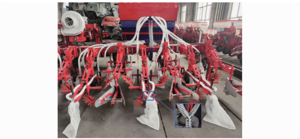
图 11 气-肥输送管合并 Fig. 11 Combined air-fertilizer conveying tube
