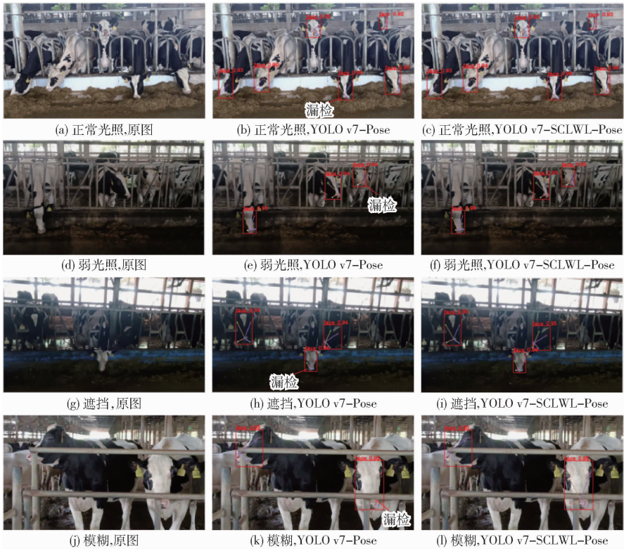
图 6 YOLO v7 - Pose、YOLO v7 - SCLWL - Pose 在不同光照和模糊条件下的检测效果 Fig.6 Detection effects of YOLO v7 - Pose, YOLO v7 - SCLWL - Pose under different conditions
