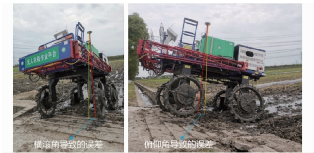
图5 车身倾斜时RTK定位坐标与车辆位置坐标误差示意图 Fig.5 Schematic of RTK positioning coordinate and vehicle position coordinate error when vehicle body was tilted
