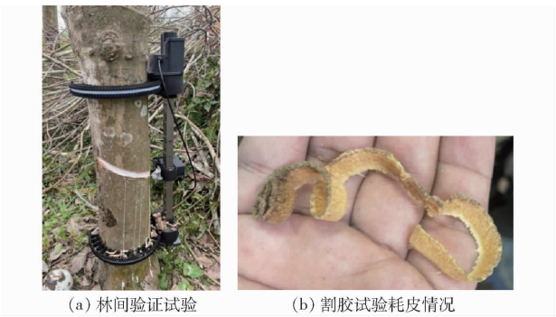
图8 林间验证试验 Fig.8 Forest test for fixed natural rubber automatic tapping machine
