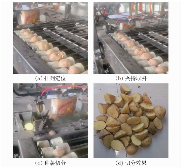
图 18 试验过程以及种薯切分效果 Fig. 18 Experimental process and effect of seed potato cutting
