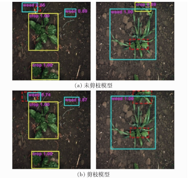
图 9 漏检现象结果 Fig.9 Results of missed inspection
