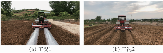
图 15 雪茄烟叶可调式苗床起垄铺膜机田间试验效果 Fig. 15 Field experimental results of cigar tobacco adjustable seed-plot ridging and film spreading machine
