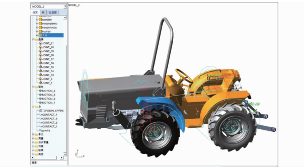
图7 轮式丘陵山地拖拉机约束模型 Fig.7 Constraint model of wheeled hilly tractor
