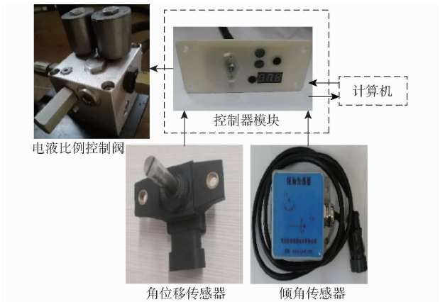
图 7 耕深电液控制系统硬件结构基本框图 Fig.7 Basic frame diagram of hardware structure of ploughing electro-hydraulic control system
