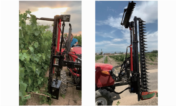
图 12 往复式葡萄剪枝机田间试验现场 Fig. 12 Field test site of reciprocating grape pruning machine
