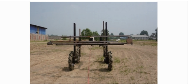
图 18 植保车直线偏移量试验 Fig. 18 Plant protection vehicle straight line offset test
