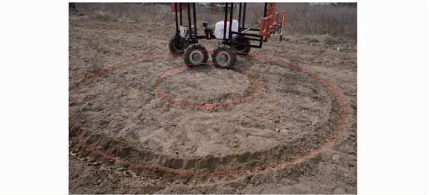
图 17 植保车转弯半径试验 Fig. 17 Turning radius test of plant protection vehicle
