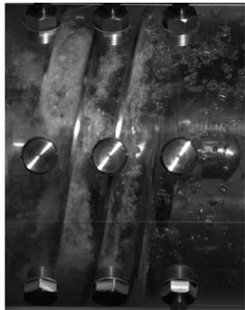
图 9 断裂后的空化区结构( \sigma = 0.014, \Phi = 0.085 ) Fig. 9 Cavity structures after breakdown ( \sigma = 0.014, \Phi = 0.085 )
