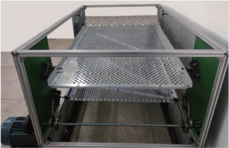
图 4 双层不平行振动筛驱动机构 Fig. 4 Driving mechanism of double-layer non-parallel vibrating screens
