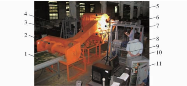
图 15 清选室流场风速测定试验台 Fig. 15 Test bench for measurement of wind velocity in cleaning room
