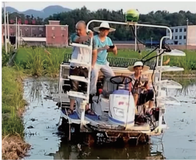
图 9 插秧机水田自动导航现场图 Fig. 9 Automatic navigation scene of transplanter in paddy field
