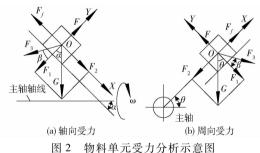
Fig. 2 Force analysis of material unit
