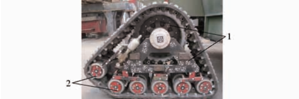
图 17 橡胶履带轮上标记点的分布 Fig. 17 Distribution of feature points on rubber track assembly
