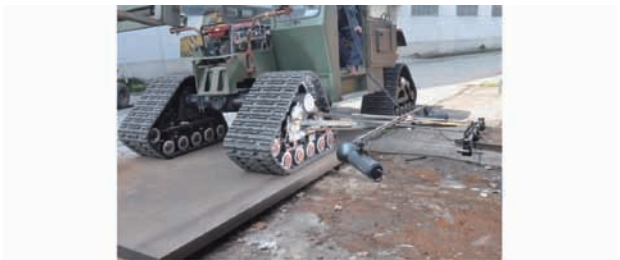
图 22 平整钢板上履带轮的测量 Fig. 22 Measurement of track assembly on flat steel plate
