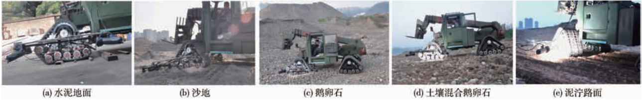
图 25 多种地形条件下履带轮的视频测量 Fig. 25 Videogrammetry of track assembly under multi-terrain conditions
