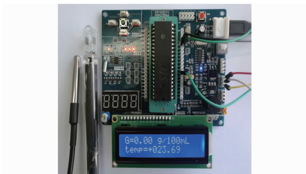
图6 豆浆总固形物含量检测仪实物图 Fig.6 Picture of total solids content detector of soybean milk
