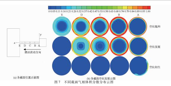
Fig. 7 Distribution of vapor volume fraction in different cross sections
