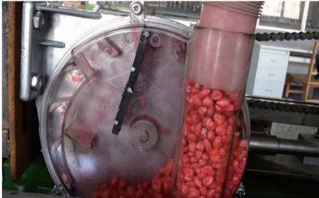
图 10 JPS-12 型排种器性能检测试验台 Fig.10 Performance test of JPS-12 seed metering device
