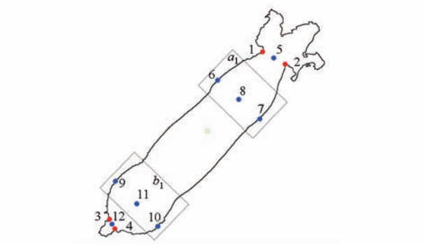
Fig. 12 Automatic detection of body measurements key points 1,2. Ear cut points 3,4. Tail root split points 5. Midpoint of neck 6,7. Measuring points for shoulder 8. Measuring points for body height 9,10. Measuring points for hip width 11. Measuring points for hip height 12. Midpoint of tail root
