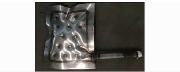
图 11 薄板水压胀型极限的验证试验 Fig. 11 Verification test of bulge forming limit for sheet
