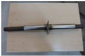
图 4 焊点机械强度测试的前处理 Fig. 4 Pretreatment of mechanical strength of welding spot
