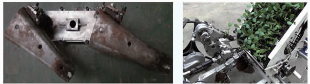
图 5 栽植机构和自主设计的全自动移栽机 Fig.5 Assembly of large spacing planting mechanism and self-designed automatic transplanting
