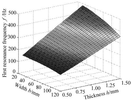
Fig. 4 Effect of width and thickness on the first natural frequency
