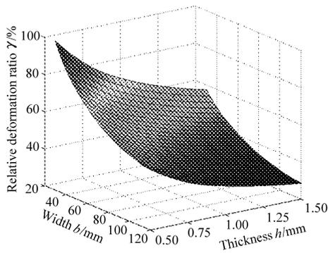
Fig. 3 Effect of width and thickness on the relative deformation ratio
