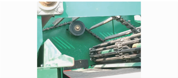
图 5 薯秧分离筛被动胶轮位置处实物图 Fig. 5 Physical image of passive rubber wheel position of sieve for separating potatoes and vines
