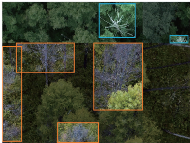
图2 Mosaic变换及LabellImg标注图像 Fig.2 Mosaic transformation and LabellImg labeling image
