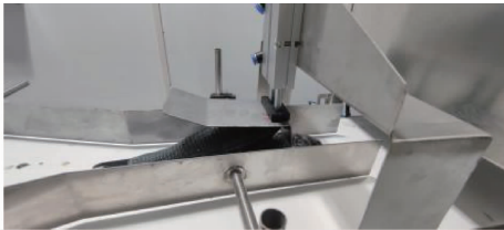
图 15 重叠鱼经过导向机构被分拨拨叉分开 Fig. 15 Overlapping fish separated by distributing fork through guide mechanism
