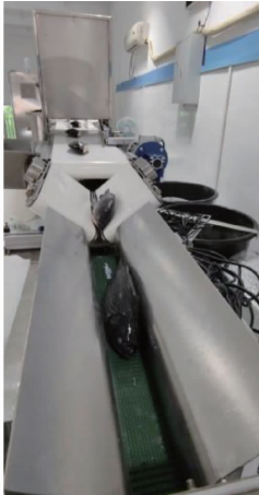
图 16 鱼体单条排列完成腹背定向工序 Fig. 16 Single arrangement of fish completes ventral-dorsal directional transportation process
