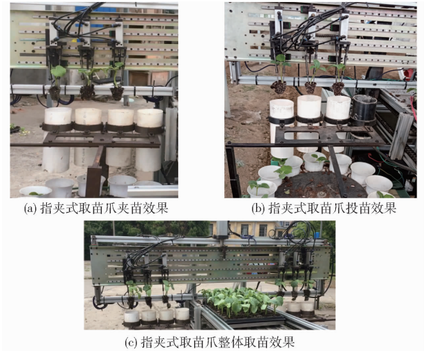
图 22 指夹式取苗爪取苗试验 Fig. 22 Picking seedling test of finger-clamping picking mechanism
