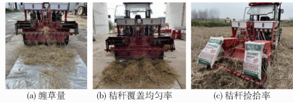
图10 性能测试试验 Fig.10 Performance test
