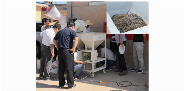
图 6 作业机试验现场 Fig. 6 Performance test of separating and cleaning machine for flax threshing material
